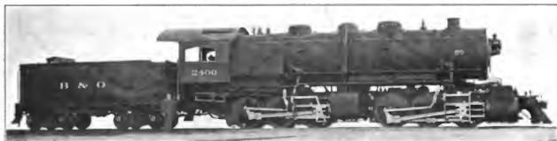
Fig. 22. Twelve-Wheel (0-6-6-0) Mallet Articulated Compound Locomotive. Built by the American Locomotive Co. for the Baltimore & Ohio. Cylinders 29 in. and 32 in. x 32 in., Working Steam Pressure 235 lbs. per sq. in., Total Heating Surface 5,585.7 sq. ft., Diameter of Drivers 56 in., Weight on Drivers 334,500 lbs., Total Weight 334,500 lbs.
